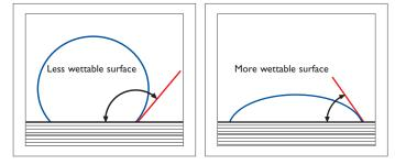
A measure of the material wettability can be defined by the contact angle between an identified liquid droplet and the mesh surface.
