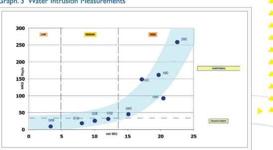
A more intuitive measure can be defined as the maximum amount of water column that a certain mesh can resist without droplet intrusion.
